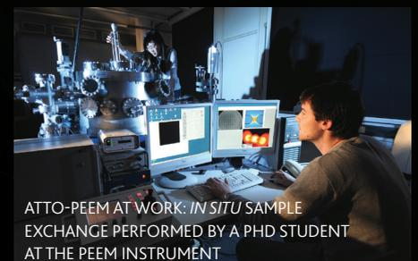
ATTO-PEEM AT WORK: *IN SITU* SAMPLE EXCHANGE PERFORMED BY A PHD STUDENT AT THE PEEM INSTRUMENT
